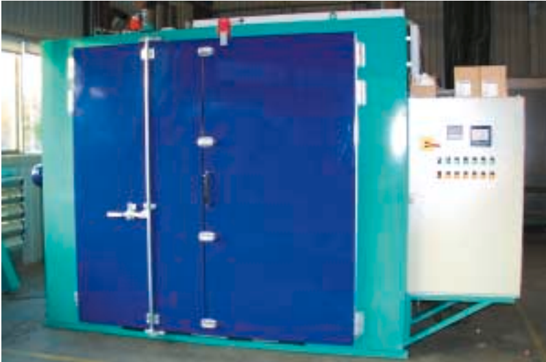
Fornax Curing Oven, custom designed T6000-S with ventilation fans on the side
